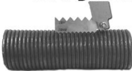
This fast and accurate stainless steel tool includes 15 saw-toothed gauges for 30 different wire sizes from .1875" to .50" for a convenient, no-miss way to measure springs in the field. Just slide the gauge over the spring for fast and accurate results. Wire sizes are stamped right on the gauge... no charts or conversions to mess with. The compact size, Go-No-Go measurement, and convenient belt sheath make this a must tool for every door installer & service technician.
