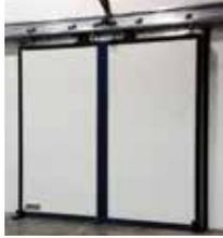
Its advanced thermal features include proprietary Flex-Panel technology for reduced downtime. Totally closed-cell EVA foam panels produce R-values ranging from R-17 (standard) up to R-40. The door is available in both sliding and bi-part designs for high-cycle applications.
