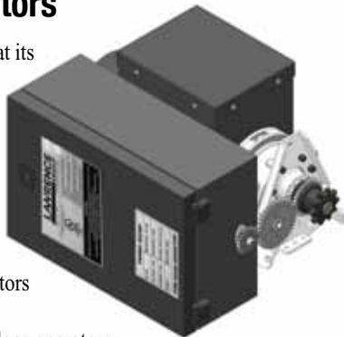
Lawrence FG Series Easy-Reset fire door operators provide automatic closing without a loss of spring tension and eliminate the need for traditional mechanical reset. Resetting is accomplished by simply reconnecting the fusible link release cable and activating the open control.
