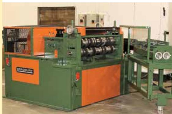
In November, Bradbury announced its new B.O.S.S. Flying Shear with Slitter. The shear runs up to 250' per minute and is capable of producing 5 slits of .048" prepainted steel, .050" aluminum, and .037" stainless steel.
