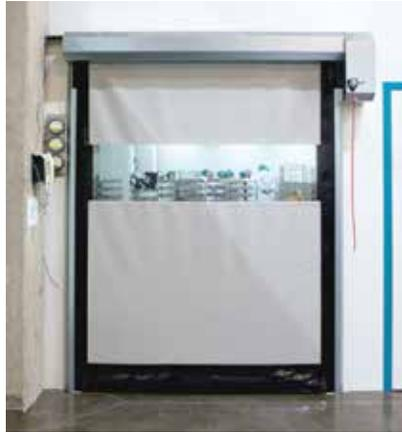
For safety, the curtain will automatically reinsert itself into the side guides if the door is hit, and an infrared photo-eye will reverse the door if an obstruction is detected. The soft bottom door curtain protects both people and products.
