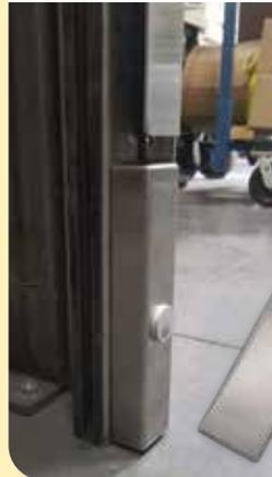
The Electronic AutoLock increases lift resistance and can withstand up to 1,200 pounds on grilles with aluminum guides and up to 940 pounds on stainless steel guides without the bottom bar lifting over the lock.
