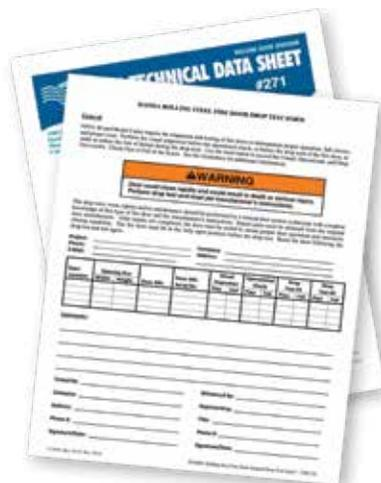
As a part of the initial installation, the annual inspection, or after repairing or retrofitting, the fire door must be drop tested twice—once to demonstrate proper operation and full closure and again to verify it was properly reset.
