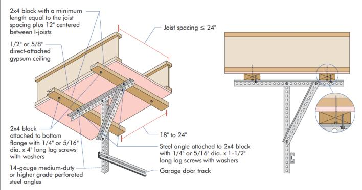
The horizontal steel angle shall be centered between the 2x4 blocks, but may be installed at any location along the length of the 2x4 blocks between I-joists. The vertical steel angle and the diagonal brace may be installed at any location along the length of the horizontal steel angle between lag screws.
