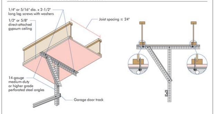
The vertical steel angle and the diagonal brace may be installed at any location along the length of the horizontal steel angle between lag screws.
