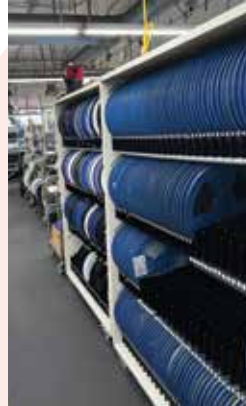
Reels of electronic components (resistors, capacitors, transistors, etc.) that are used with the surface mount technology insertion machine.
