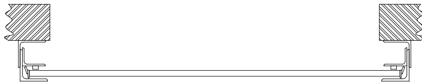
Figure 3 No Wind Load With Windlocks
