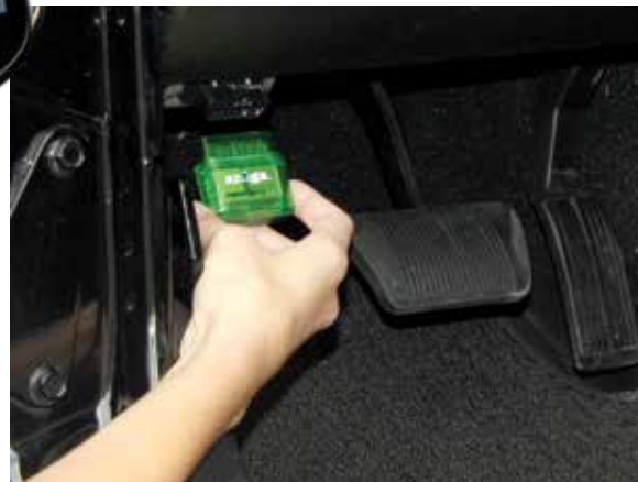
INSTALLED: The GPS tracking device is typically installed under the truck's dashboard in the OBD-II port.
