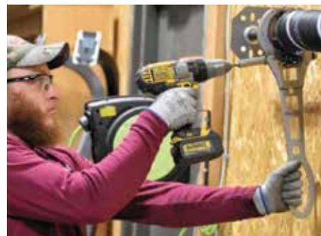
The tool eliminates the need for winding bars and reduces the time needed to wind springs. Other benefits of spring-winding tools are featured on pp. 58-62. [www.surewinder.com](http://www.surewinder.com)
