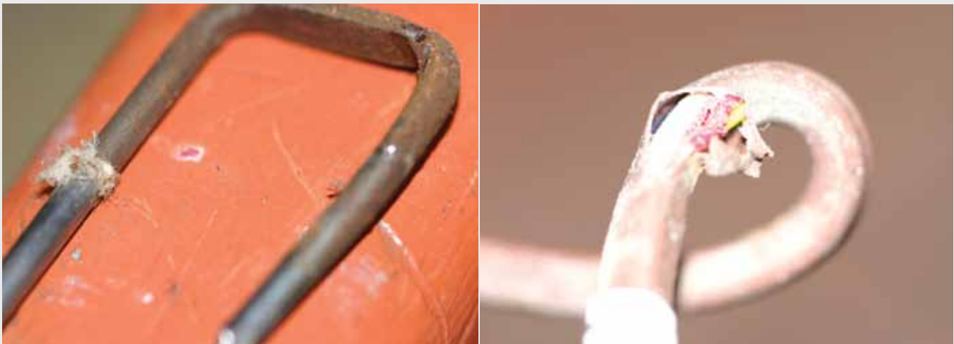
BARE METAL STAPLE: This staple is believed to have cut through this wire, causing the door to open when Parker handled it. (Photo used with permission.)
