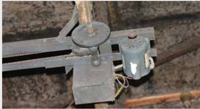
THE OPERATOR INVOLVED: This operator, thought to be 30 years old, is missing its belt because it had burnt off during the accident. (Photo used with permission.)
